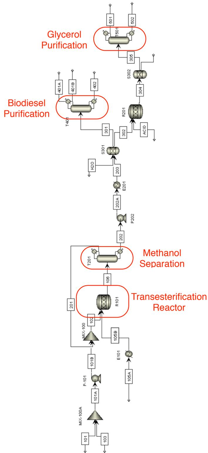
**Figure 2.3:** Simplified flow chart diagram showing the main processing units of the the alkali-catalyzed process for biodiesel production.
