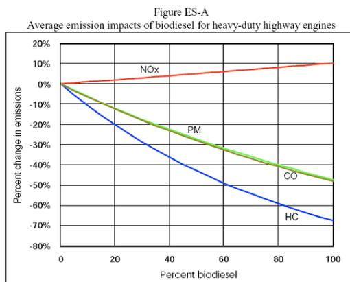
Figure 3.1: EPA estimates of average emission impacts of biodiesel for heavy-duty highway engines.
