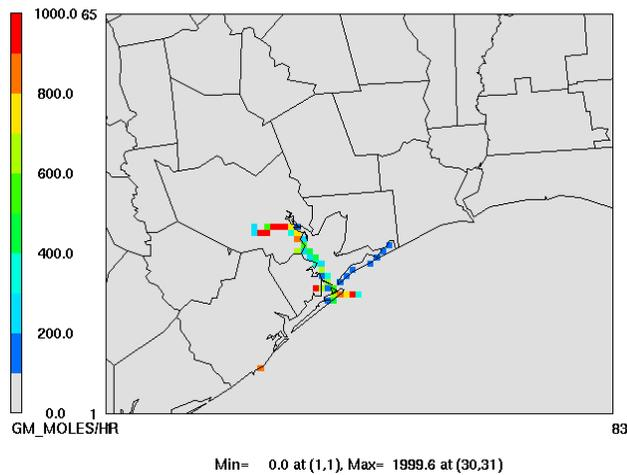
Figure 3.10: NO<sub>x</sub> emitted from ships diesel engines
