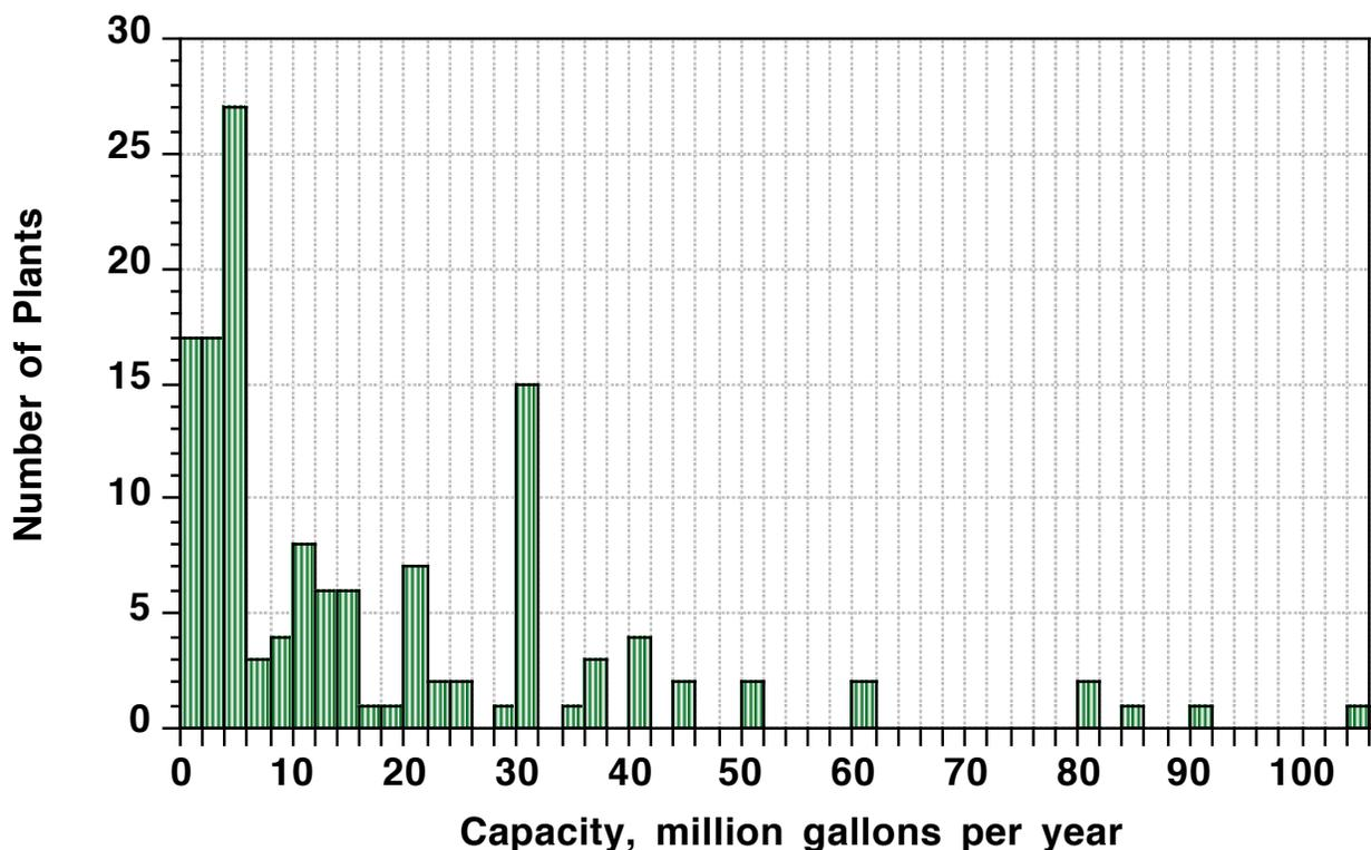
Figure 2.2: Histogram of the production capacities of US biodiesel plants.
