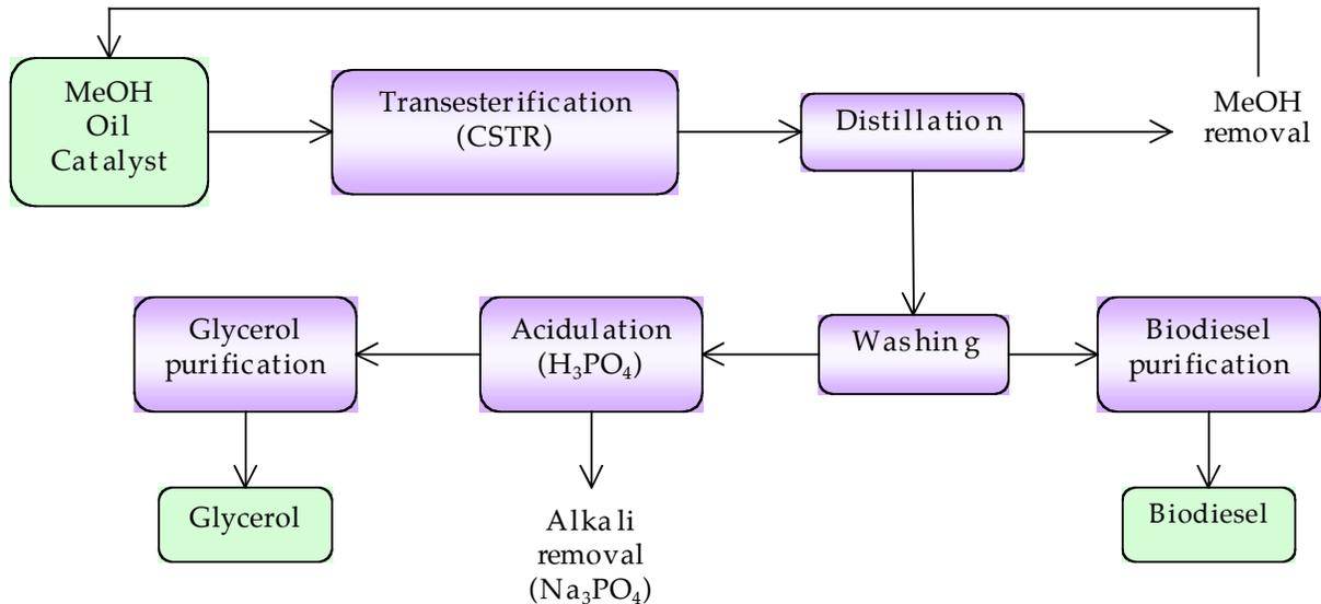
Figure 2.1: Basic steps of alkali-catalyzed process for biodiesel production.
