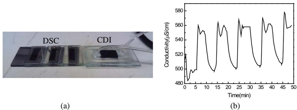
Figure 1. Desalination curve of a CDI driven by 2V solar module for 5 cycles.
