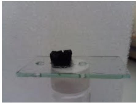
Figure 3. 1 centimeter long multi-walled carbon nanotube forest transferred to a transparent conductive glass. PDMS has been used as binder and the adhesion is strong. This technique gives much larger carbon loading amount comparing to other carbon nanotubes based electrode preparation methods do.
