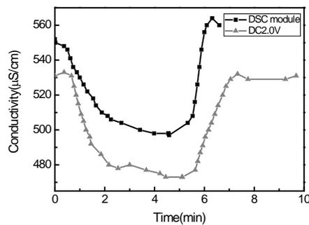
Figure 2. Comparison of desalination curve for the same CDI device driven by DSC module and DC 2V source separately.
