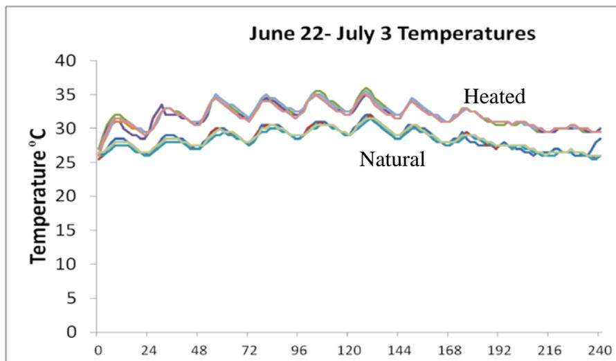
**Figure 1:** Temperature dynamics in four heated and four tanks with natural temperature dynamics for a 240 hrs period.
