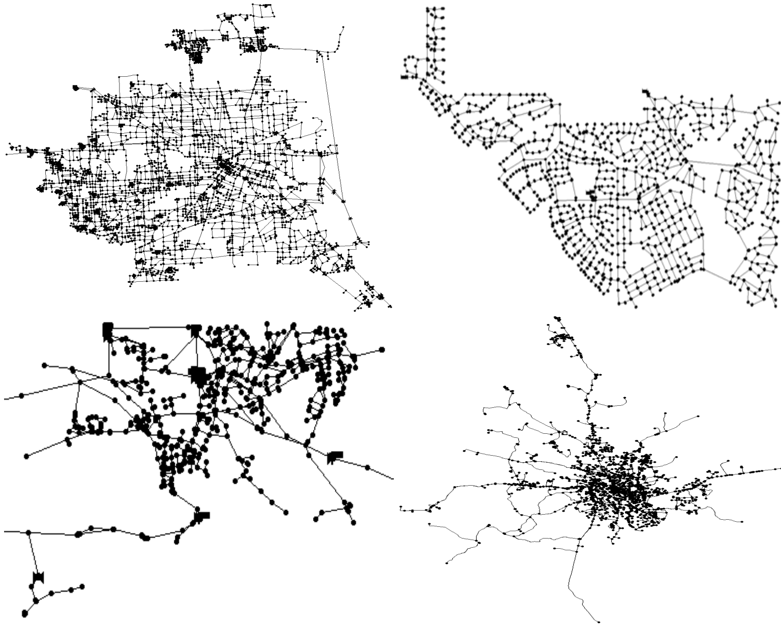
Figure 1 EPANET view of City of Houston COH (top left), Colorado Springs CS (top right), Yorkshire Water Richmond YWR (bottom left), Kumasi KUM (bottom right)
